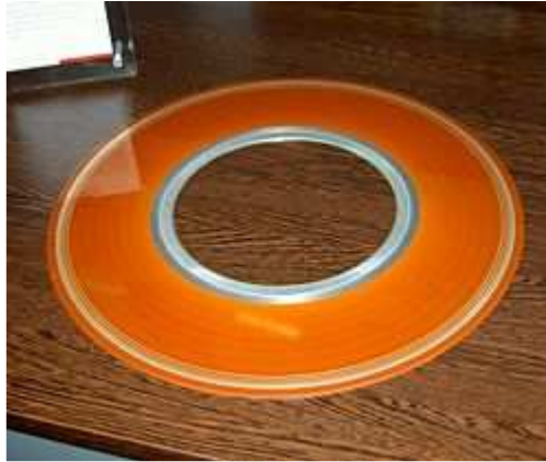
IBM RAMAC disk showing head crash damage
